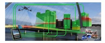
To ensure that the **positioning**, and also information from other gauges recording **acceleration**, **strain** and **temperature** from the monitored buildings can reach the base station, a **gateway-PCCDN** tool for communication will be developed in this work that will provide redundancy at situations of access network unavailability by utilizing multiple and different access interfaces, e.g., GSM, UMTS.
