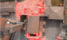
Figure 9. UAV image taken after the 2012 Mirabello earthquake (left); damaged regions mapped by our method in red mask (right)
