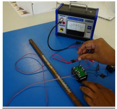
Figure 3. Bridge Balancing with Adjustment Potentiometer
