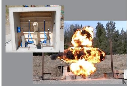
Figure 6. Left: One of the test structures with instrumentation inside. Right: One of the explosives test with the test structure to the left and the blast to the right.
