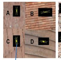
Histogram of gradient orientation pattern of non-damaged region
