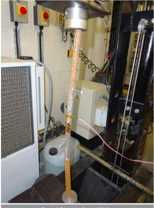
Figure 4. Rebar at a Strain of 2040µɛ
