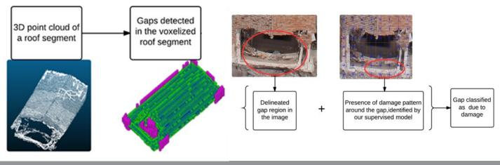
Figure 10. Detection of Structural Gaps
