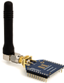
Figure 32-802.15.4/ZigBee Pro module
