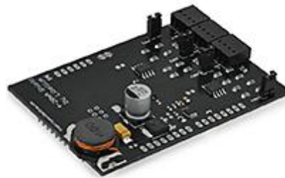
Figure 34-4mA/20mA current loop module
