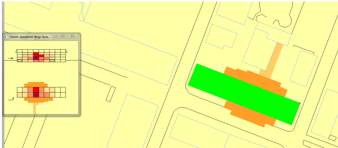
Figure 9: An example of output from the VEBE code where a high explosive charge has been detonated on the first floor of a building type M1TN. To the right it is shown different zones outside the building where debris is falling (dark orange) or thrown (light orange). The small figure to the left shows the building divided into construction units (volumes divided by load-bearing walls) with different damage zones inside the building (solid red – floor collapse zone, red grid – wall collapse zone, red hatched – crack zone and red dot pattern - shake zone).
